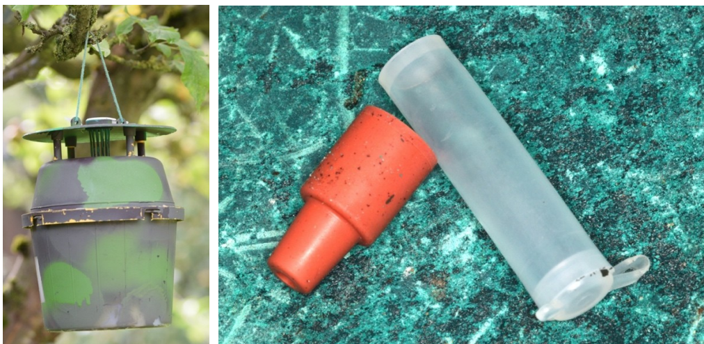
Figure 3. A camouflaged pheromone lure trap (left) and rubber bung and plastic vial lures impregnated with the pheromones (right).
